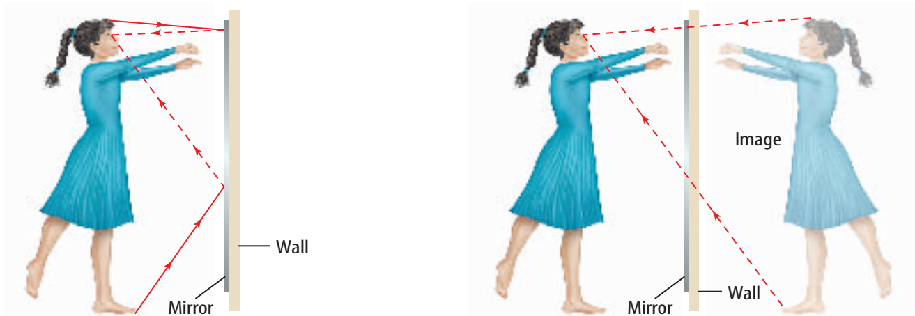
A Light rays that bounce off a person strike the mirror. Some of these light rays are reflected into the person's eye. B The light rays that are shown entering the person's eye seem to be coming from a person behind the mirror.
